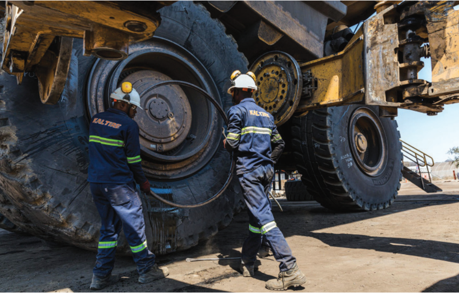
As part of an overall maintenance plan, a tire management program like Kal Tire's TOMS can be implemented to establish and maintain benchmark tire care strategies including inspection frequency and guidelines, tire rotations, target cold pressures and rim non-destructive tests (NDTs).
